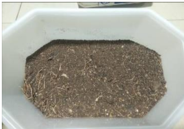
Figure 4. Powdered Banana Peel (Saba Peel) Used as an Adsorbent for the Nutrient of Wastewater
