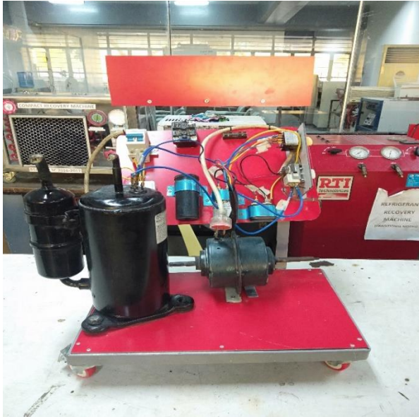
Figure 4. Shows the Actual Front View of the Developed Prototype For Domestic Air-Conditioning Training Equipment
