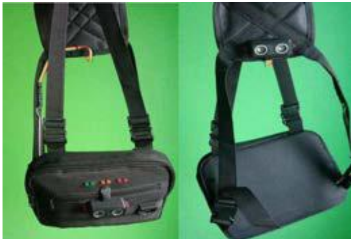
Figure 4. Chest-Rig Embedded Social Distancing Sensor Using Arduino
