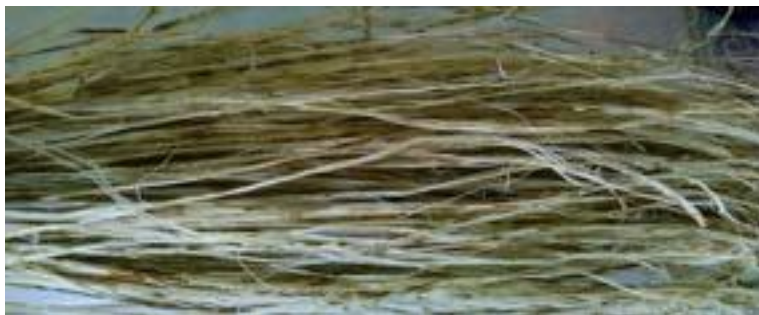
Figure 4: The Moringa Fruit Skin Fibers after Soaking and Air Drying
